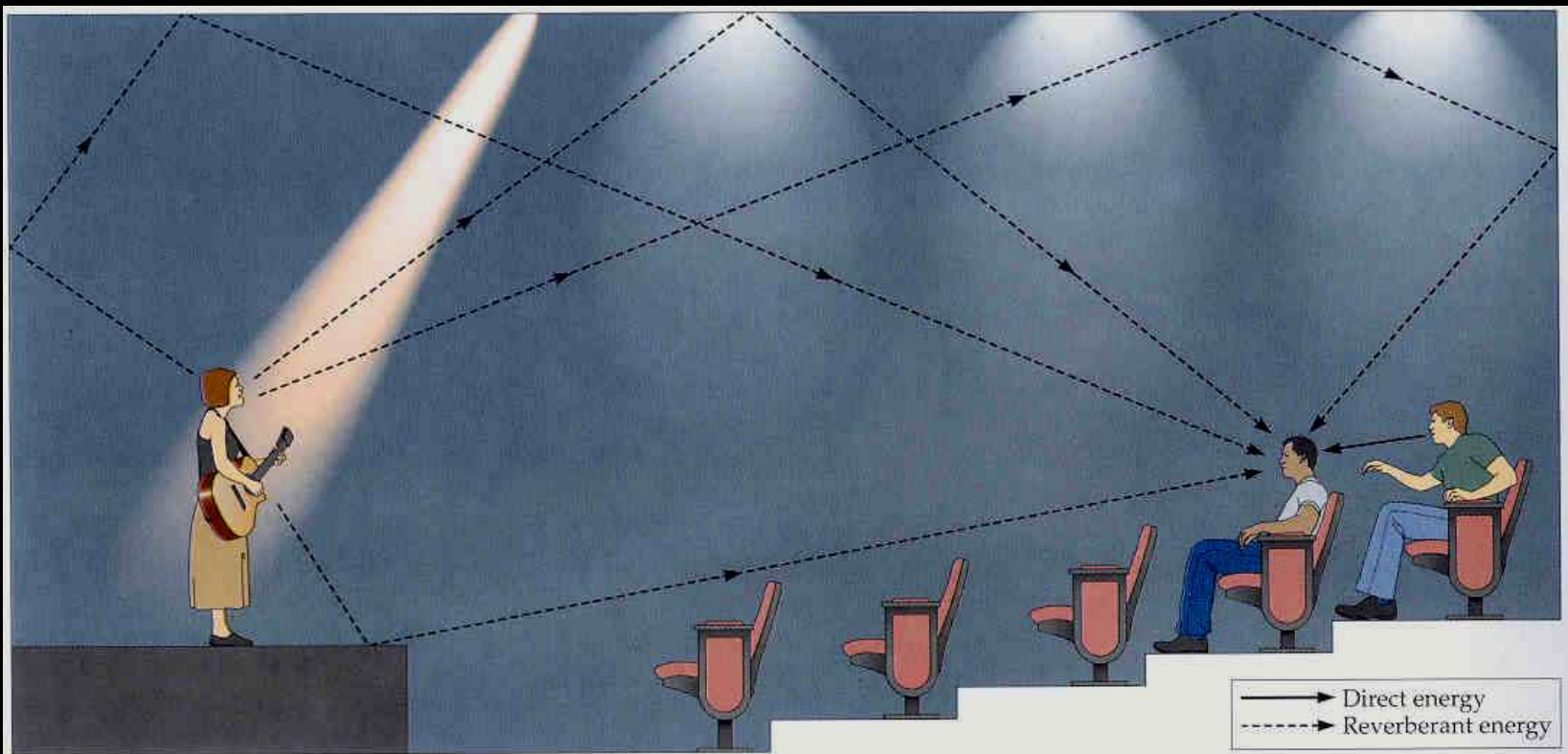
FIGURE 10.11 The relative amounts of direct and reverberant energy coming from the listener's neighbor and the singer will inform him of the relative distances of the two sound sources.
