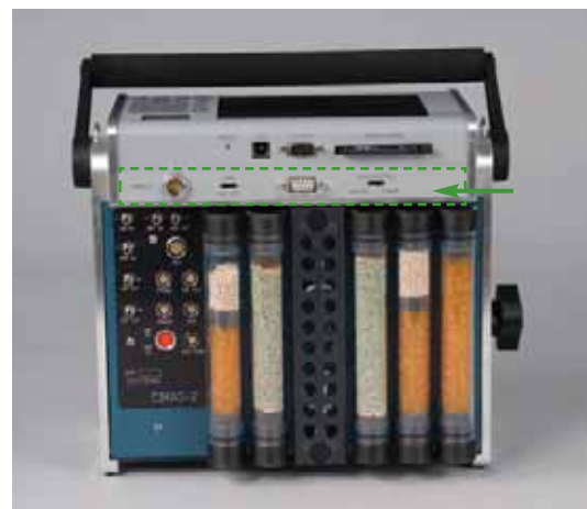
The CIRAS-2 shown above with integral Chlorophyll Fluorescence Module (CFM) signal conditioning interface.
