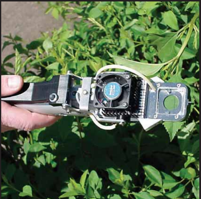
PLC6 (U) Automatic Universal Leaf Cuvette
