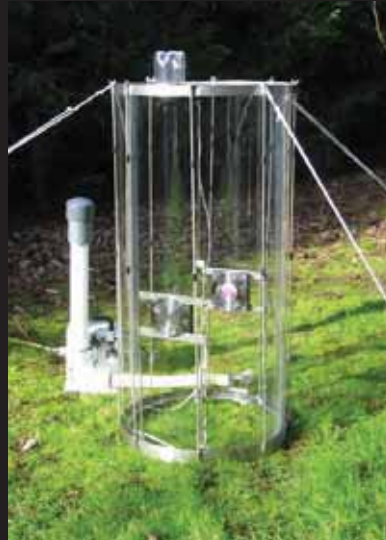
CPY-3 chamber for tall vegetation. Our Control Interface Module (CIM) with required air supply unit is also shown in the background.
