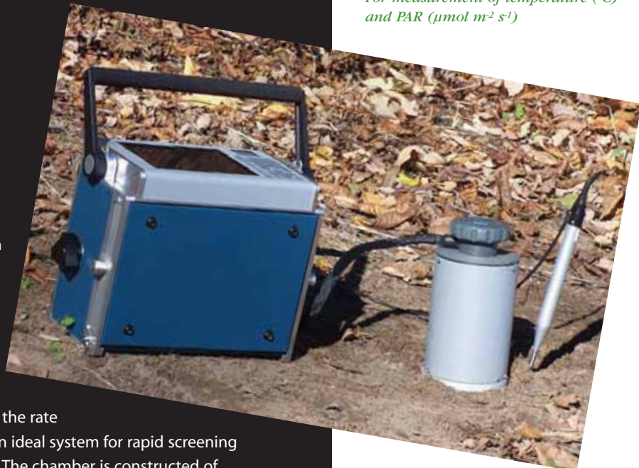
The CIRAS-2 shown with the SRC-1 Soil Respiration Chamber and STP-1 Soil Temperature Probe.
