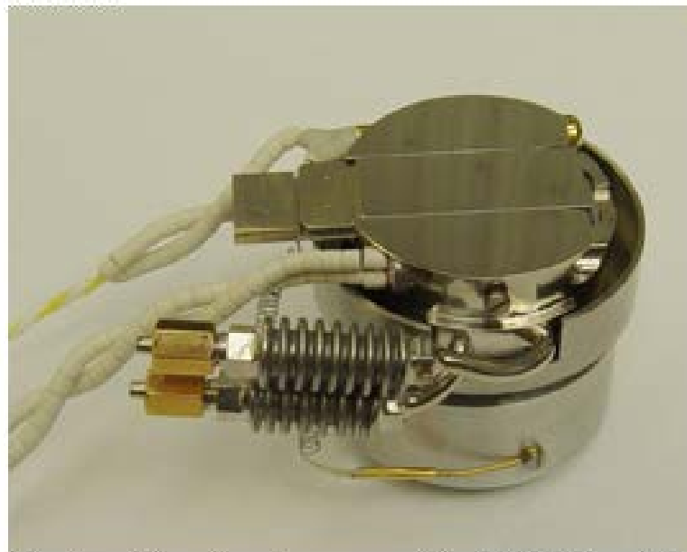
Cooling / heating stage module -185°C to +400°C
