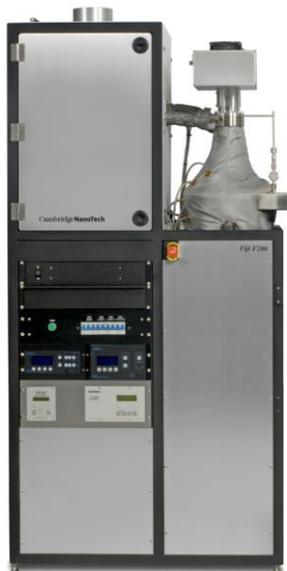
The Fiji F200 ALD process chamber, heater and trap geometries have been optimized for ALD processing: the hyperboloid chamber geometry combined with the paraboloid substrate heater creates a laminar precursor and remote plasma generated radical flow. This design optimizes deposition uniformity and minimizes cycle time and precursor use.
