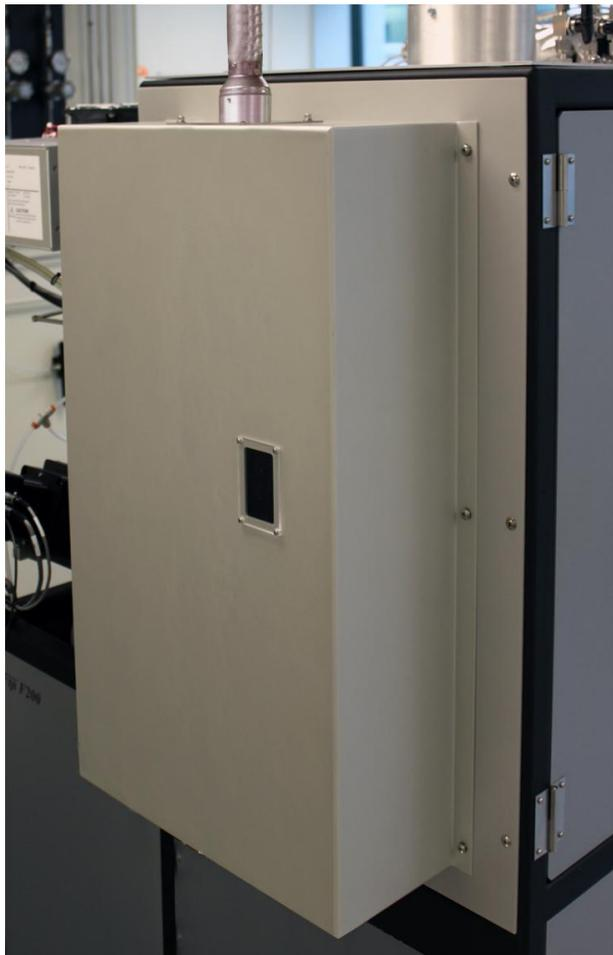
**Figure 1: Fiji Ozone Generator Installed on System**
