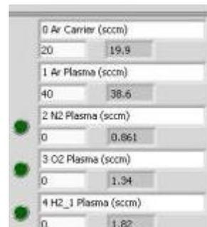
The MFC setpoints can also be set programmatically with the “flow” recipe command. The flow command takes two arguments. The # argument refers to the MFC number. The value argument is the desired flowrate in sccm.
