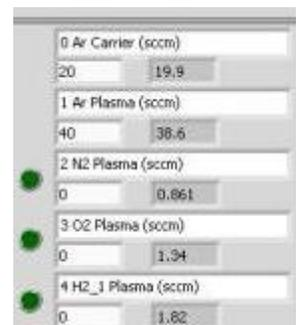
The MFCvalve command takes two arguments. The # argument is the MFC number and value is either 0 for closed or 1 for open.
