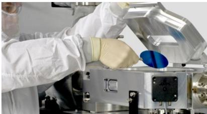
After loading a substrate, the loadlock chamber is closed then pumped down. After reaching the appropriate differential pressure between the loadlock and process chamber, the main gate valve between the loadlock and process chamber is opened. The substrate carrier is then manually transferred via a magnetically-coupled transfer arm onto the heated chuck in the process chamber.
