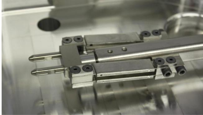
*'End effector' of transfer arm in a raised position when transfer arm is rotated.*
