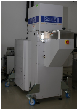
Oxford Instruments, PlasmaPro 100 - reactive ion etching
