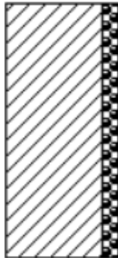
Remove cupric oxide overlayer.
