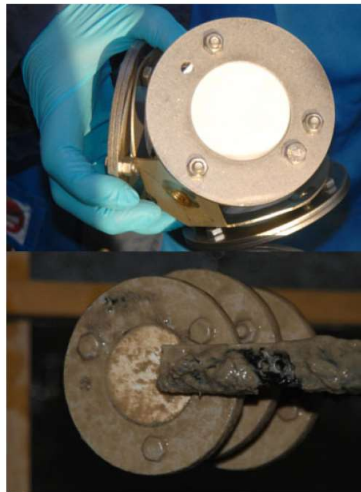
Fig. 1. Differences in polar organic chemical integrative samplers (POCIS) fouling from different deployment environments. Very lightly fouled POCIS (upper picture) deployed in the Norwegian Sea (~200 km offshore) for 42 d and moderately fouled POCIS (bottom picture) from wastewater treatment works after 14 d exposure. [Color figure can be seen in the online version of this article, available at wileyonlinelibrary.com .]
