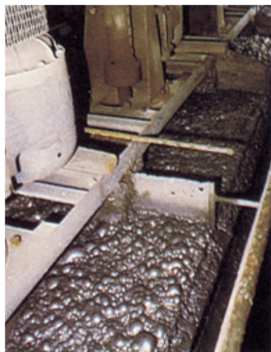
Figure 22-11 A copper ore being enriched by flotation.
