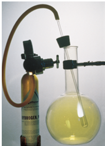
Figure 6-5 Hydrogen, \text{H}_2 , burns in an atmosphere of pure chlorine, \text{Cl}_2 , to produce hydrogen chloride.
