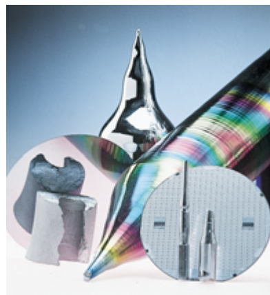
Various samples of elemental silicon. The circle at the lower right is a disk of ultrapure silicon on which many electronic circuits have been etched.
