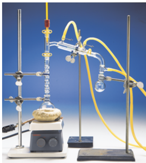
Figure 14-13 A fractional distillation apparatus. The vapor phase rising in the column is in equilibrium with the liquid phase that has condensed out and is flowing slowly back down the column.
