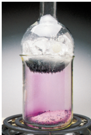
Figure 13-16 Sublimation can be used to purify volatile solids. The high vapor pressure of the solid substance causes it to sublime when heated. Crystals of purified substance are formed when the vapor is deposited to form solid on the cooler (upper) portion of the apparatus. Iodine, \text{I}_2 , sublimates readily. \text{I}_2 vapor is purple.
