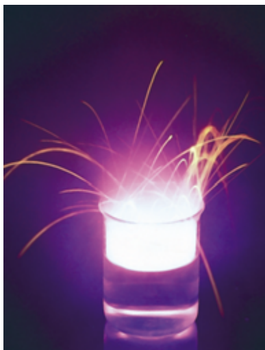
Figure 4-4 Potassium, like other Group IA metals, reacts vigorously with water. For this photograph, the room was completely dark, and all of the light you see here was produced by dropping a small piece of potassium into a beaker of water.
