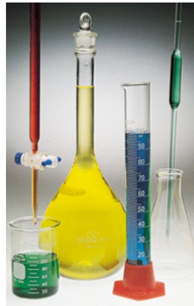
Figure 1-13 Some laboratory apparatus used to measure volumes of liquids: 150-mL beaker ( bottom left , green liquid); 25-mL buret ( top left , red); 1000-mL volumetric flask ( center , yellow); 100-mL graduated cylinder ( right front , blue); and 10-mL volumetric pipet ( right rear , green).
