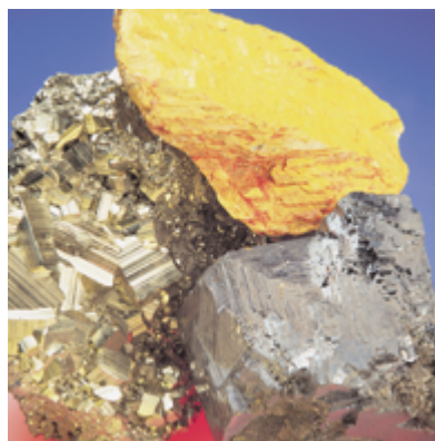
Some sulfide minerals: iron pyrite (fool's gold), \text{FeS}_2 ; black galena, \text{PbS} ; yellow orpiment, \text{As}_2\text{S}_3 .
