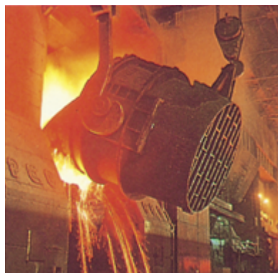
Molten steel is poured from a basic oxygen furnace.
