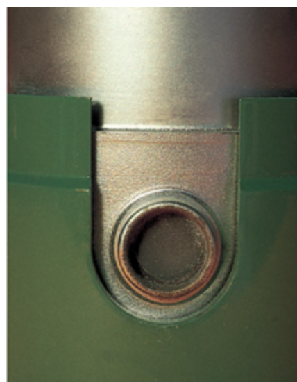
A laboratory X-ray tube ( left ) and a close-up view of one of its windows ( right ). The windows are made of beryllium metal.
