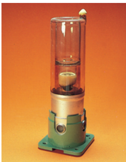
A laboratory X-ray tube ( left ) and a close-up view of one of its windows ( right ). The windows are made of beryllium metal.
