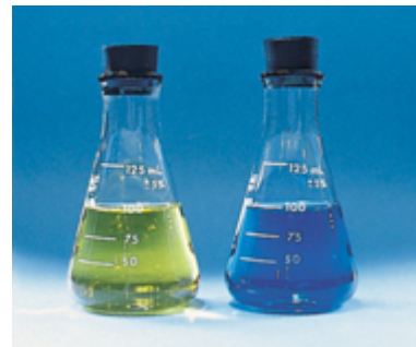
Bromthymol blue indicator is yellow in acidic solutions and blue in basic solutions.
