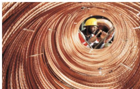
Copper is drawn into wire, which is then collected into cables for use as an electric conductor.
