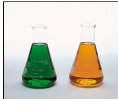
\text{Cr}_2(\text{SO}_4)_3 is green in acidic solution. \text{K}_2\text{Cr}_2\text{O}_7 is orange in acidic solution.
