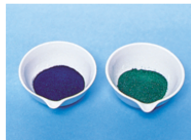
Figure 25-2 The dichlorobis(ethylenediamine)cobalt(III) ion, [Co(en) 2 Cl 2 ] + , exists as a pair of cis-trans isomers. Ethylenediamine is represented as \overset{\curvearrowright}{\text{N}} \text{---} \text{N} . Cis -dichlorobis(ethylenediamine)cobalt(III) perchlorate, [Co(en) 2 Cl 2 ]ClO 4 , is purple. Trans -dichlorobis(ethylenediamine)cobalt(III) chloride, [Co(en) 2 Cl 2 ]Cl, is green.
