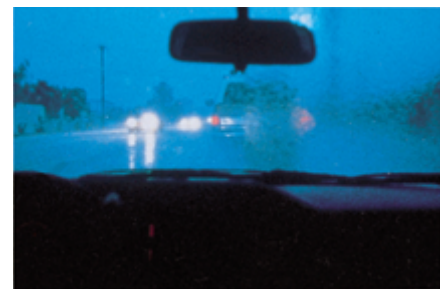
Coating glass with a silicone polymer greatly reduces the adhesion of water to the glass. The left side of each glass has been treated with Rain-X, which contains a silicone polymer. Water on the treated side forms droplets that are easily swept away.
