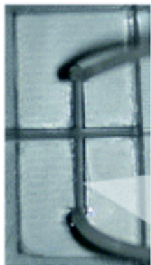
F. Circular channel assembly from two PDMS slabs
