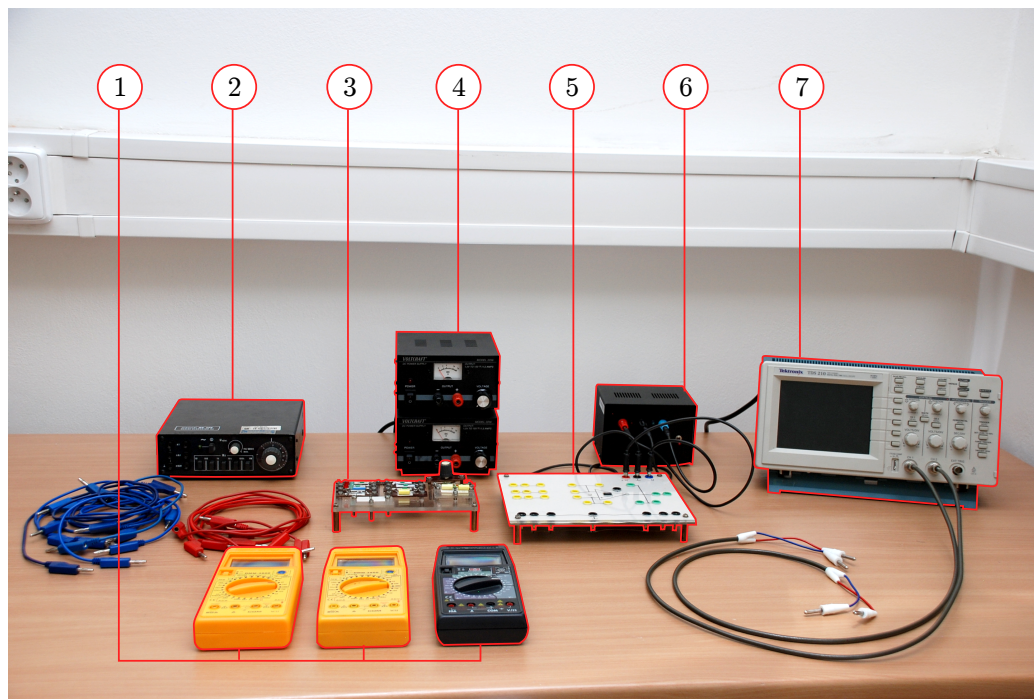
Figure 2: Operational amplifier setup: 1. Multimeters. 2. AC power supply. 3. Different electrical components. 4. DC power supplies. 5. Circuit board with the operational amplifier. 6. Power supply. 7. Oscilloscope.
