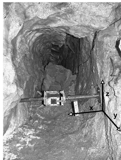
Fig. 10. The TM71 deformer installed across the monitored fissure in the cave Na Pomezí (site P1).
