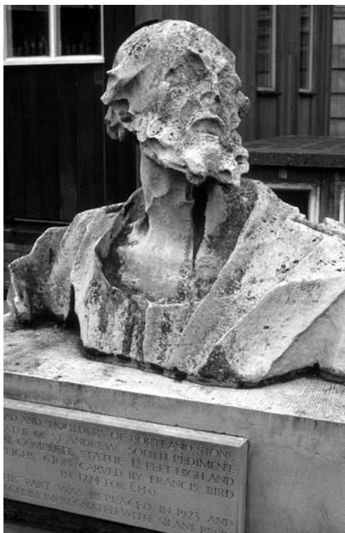
Plate 6.5 A bust of St. Andrew, removed from St. Paul's Cathedral because of accelerated decay. (Photograph by Heather A. Viles)
