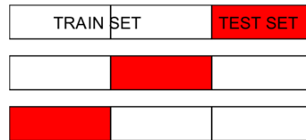
Figure 5. A 3-fold cross-validation scheme: each of the folds is used once and only once as validation set (the red block).
