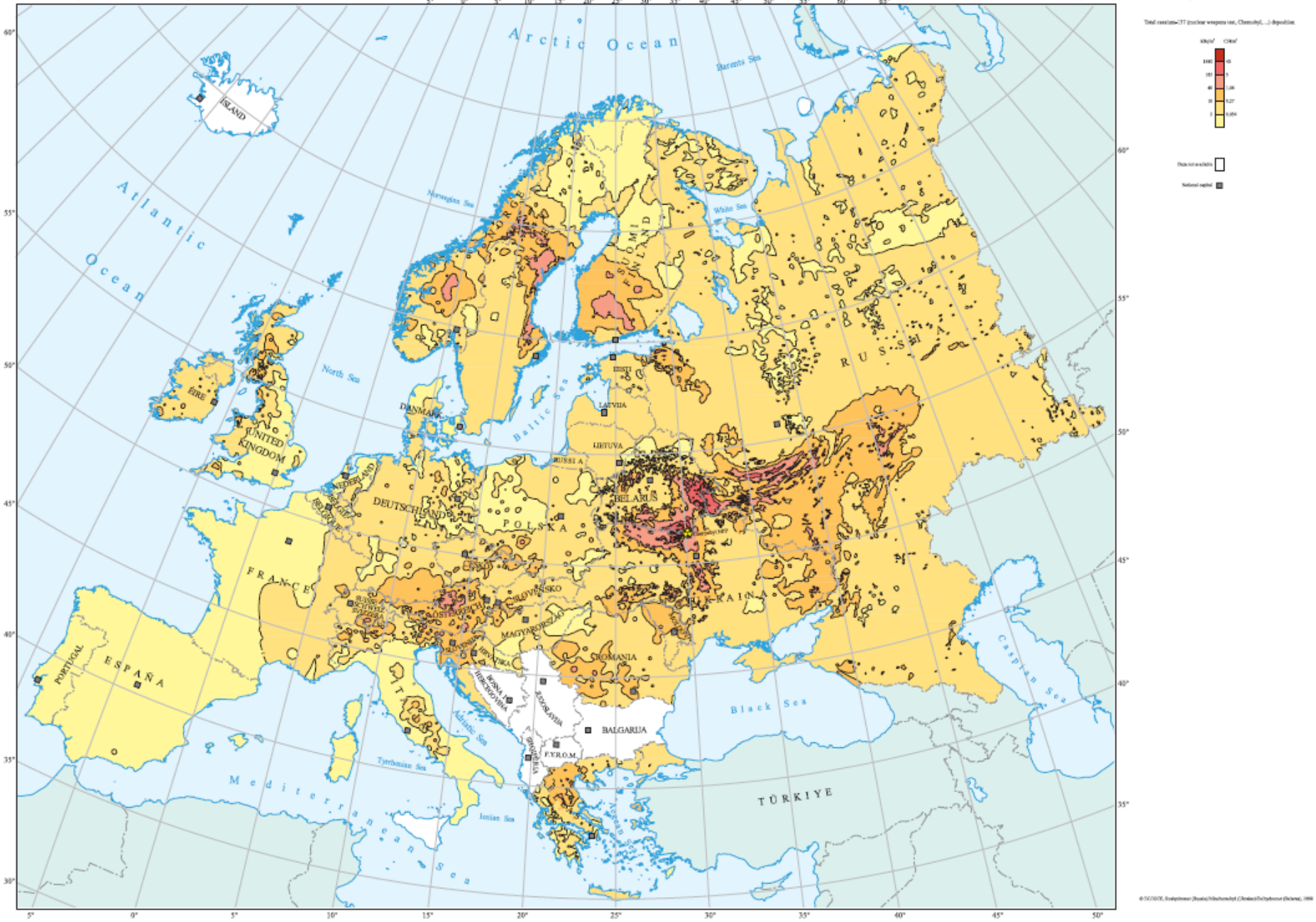
Figure XI. Surface ground deposition of caesium-137 released in Europe after the Chernobyl accident [D13].
