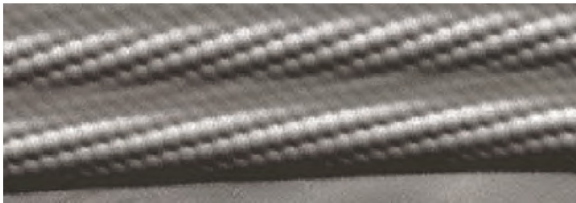
Fig. Image of two neighboring chiral SWNTs within a SWNT bundle as seen using high-resolution scanning tunneling microscopy
