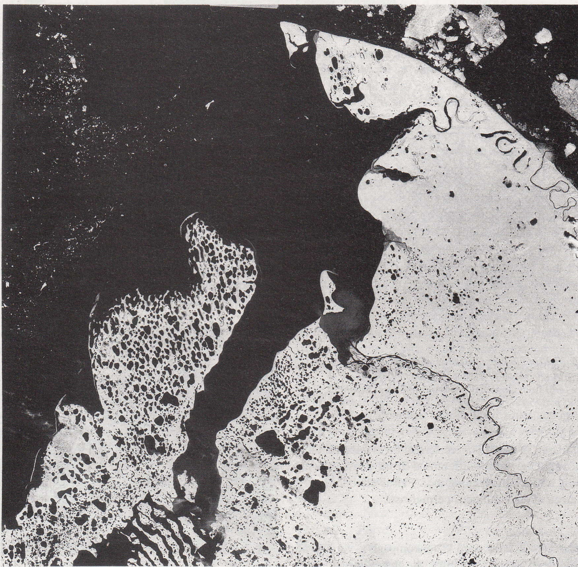
Fig. 12.14 Thaw lakes in the Tuktoyaktuk Peninsula which lies within the continuous permafrost zone of the Northwest Territories, Canada. The area shown is about 180 km across. (Landsat image courtesy R. S. Williams Jr)
