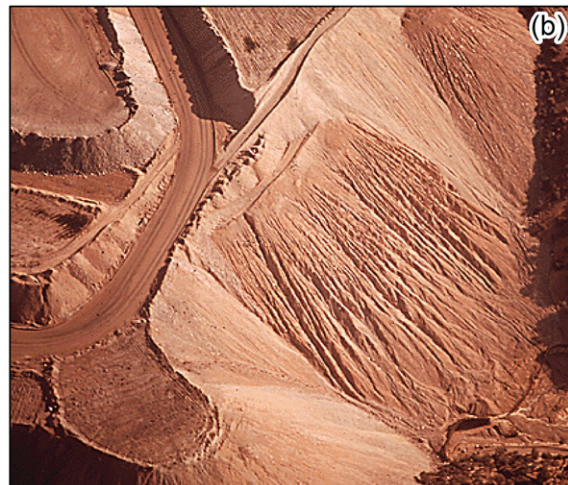
Fig. 3. Surface mining in the Rhineal-Pfalz region (Germany) (photo by G. Sofia) (a) and erosion of tailing piles in a copper mine (Agency, U.S.E.P., 1972).
