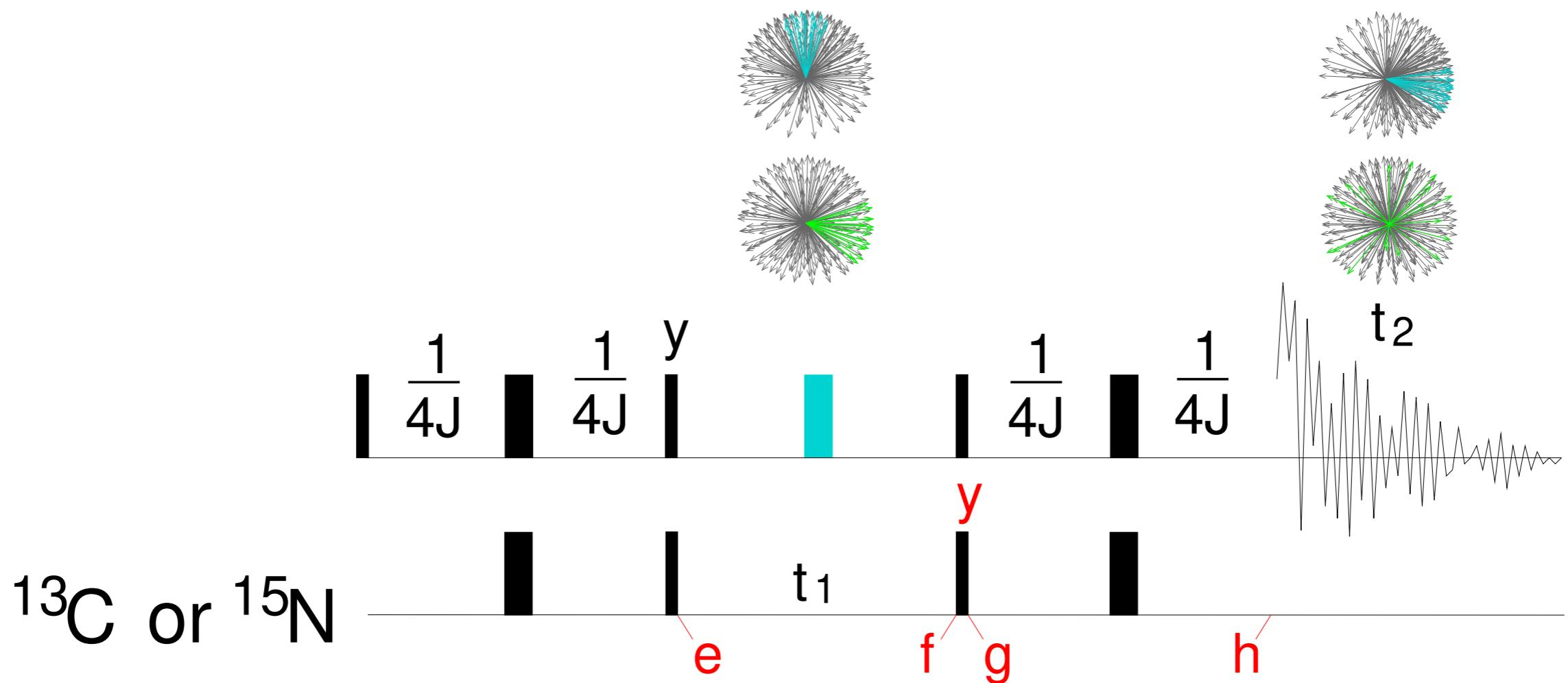
BLOCK 3: TWO  $90^\circ$  PULSES, PHASE  $y$  (<sup>13</sup>C or <sup>15</sup>N)
