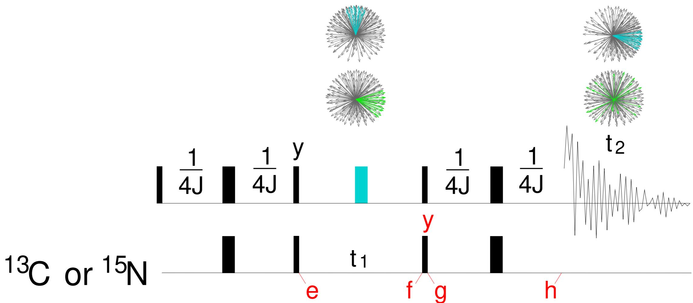
BLOCK 3: TWO  $90^\circ$  PULSES, PHASE  $y$  ( $^{13}\text{C}$  or  $^{15}\text{N}$ )
