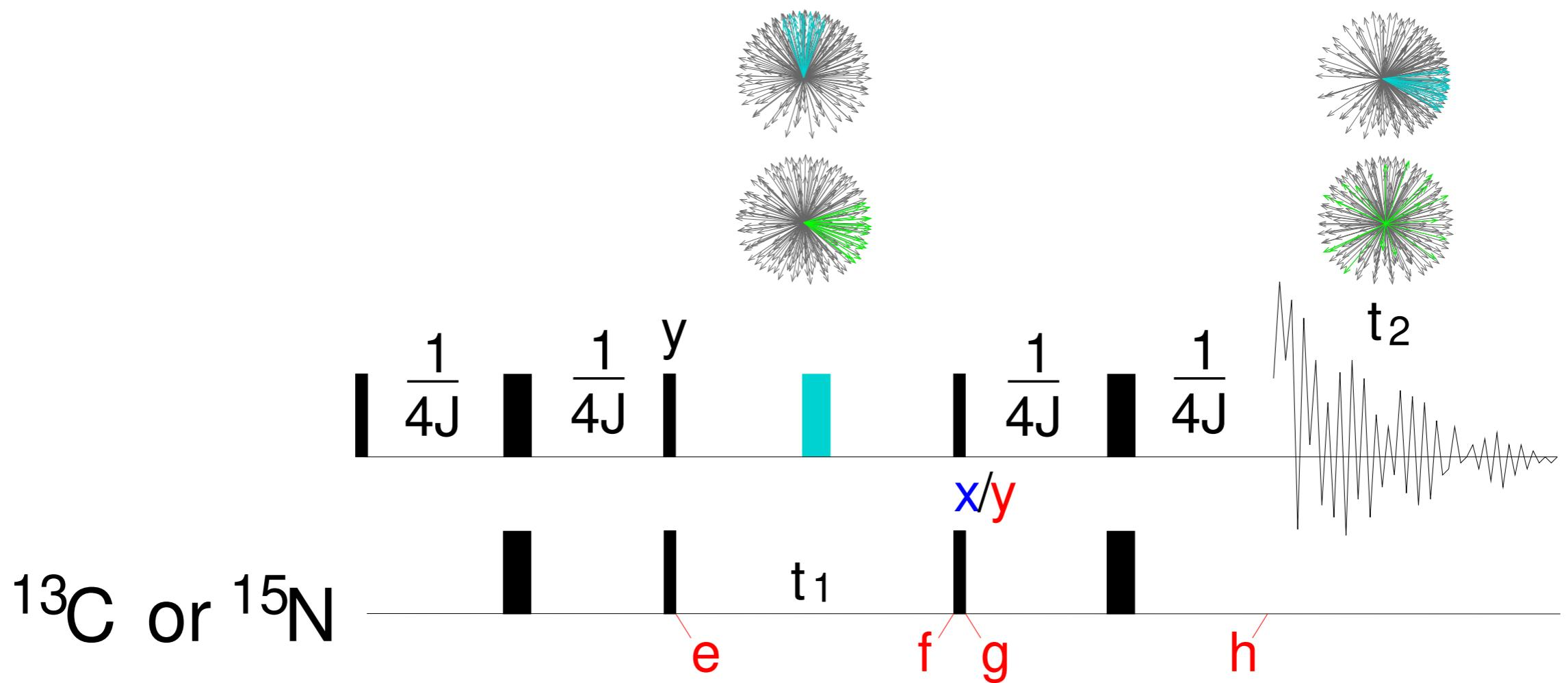
BLOCK 2: DECOUPLING ECHO, INCREMENTED  $t_1$
