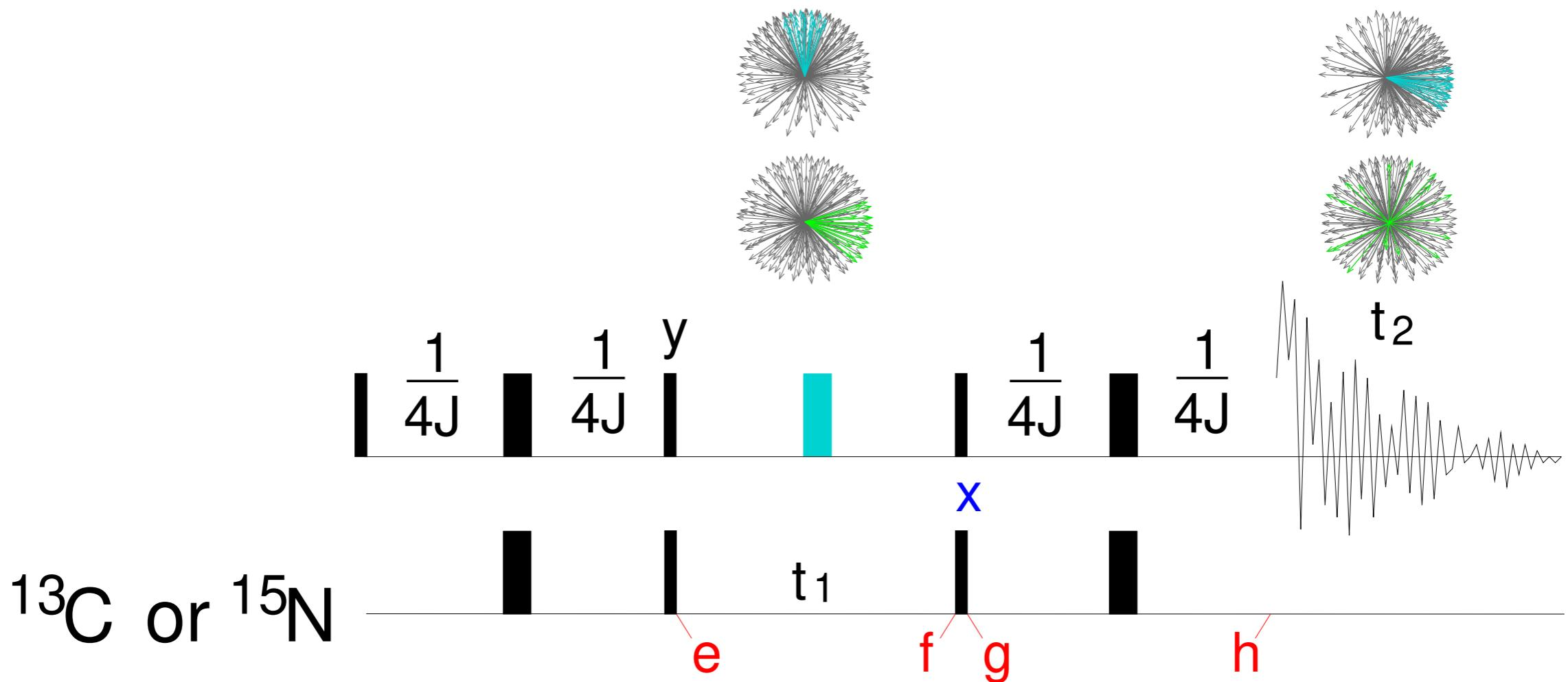
BLOCK 3: TWO  $90^\circ$  PULSES, PHASE  $\times$  ( $^{13}\text{C}$  or  $^{15}\text{N}$ )
