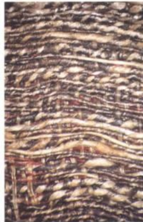
Fig. 5 Gew 370: Silver coated mem- brane strip wound around a linen core
