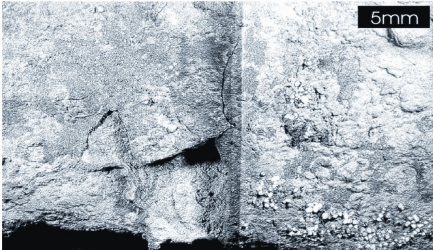
Fig. 6. Liquid film (ethanol) on the surface also removes silica grains; left : laser cleaned ( \lambda = 1064 nm) with ethanol liquid film; right : laser cleaned ( \lambda = 1064 nm) without ethanol liquid film
