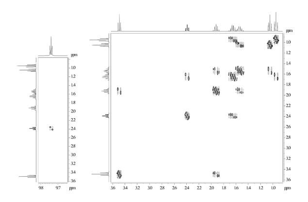
4. Try to identify resolved <sup>1</sup>H signals of a diterpenoid-lactone based on 1D NMR spectrum and NOESY correlations.
