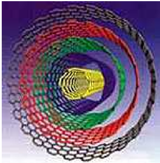
■ MWCNT interlayers spaced 0.34 nm
