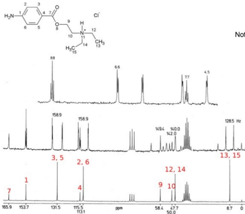
1D  $^{13}\text{C}$ -NMR 3, *b* - zoom of right region, *a* - full decoupled spectrum
