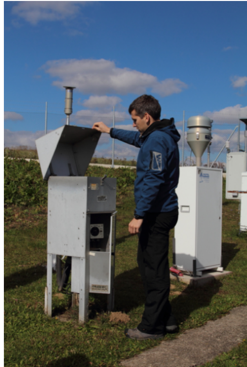
high volume active sampler PS1 Thermo and Digital DH-77 (2011) active sampling in Czech Republic (10/1988)
