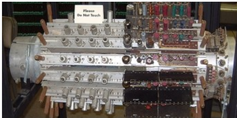
Mercury memory of UNIVAC (1951)
