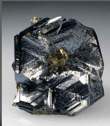
Polybasite, [Ag_9CuS_4] [(Ag,Cu)_6(Sb,As)_2S_7] , Chispas Mine, Arizpe, Mun. de Arizpe, Sonora, Mexico. Overall specimen is 3 cm across. Wendell Wilson photograph.
