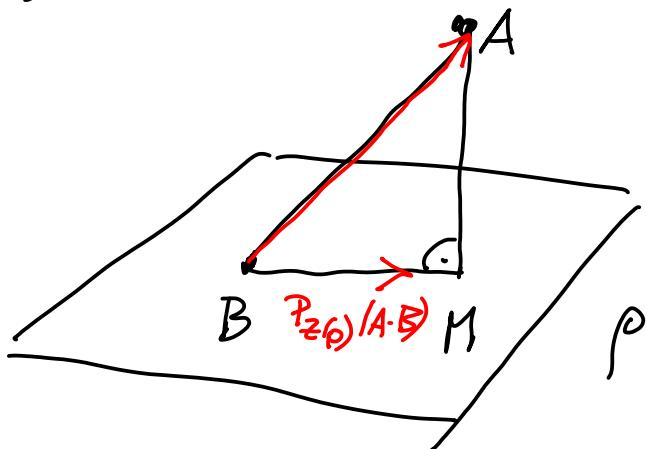
$$\begin{aligned} \underline{\underline{M}} &= B + P_{Z(\rho)}(A-B) = \\ &= [3, -2, 1, 5] + (0, 5, -7, -6) = \underline{\underline{[3, 3, -6, 1]}} \end{aligned}$$
