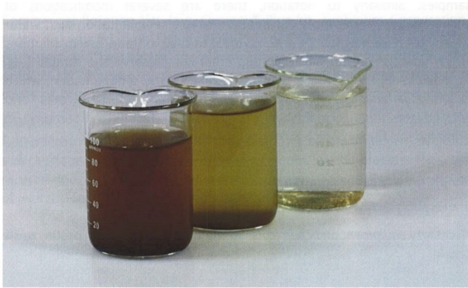
Fig. three stages of gravity sedimentation technique; initial stage on left, final stage with clearly separated sediment on right.
