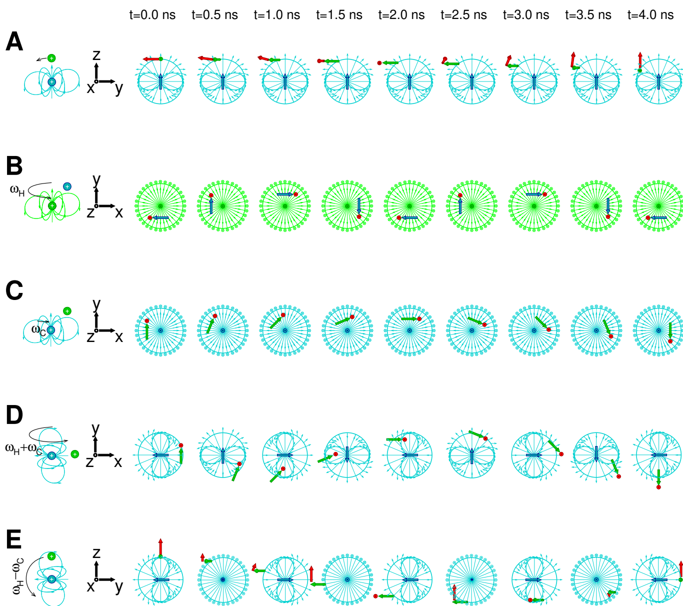
Figure 8.2: Illustration how random molecular motions resonating with five characteristic frequencies affect \vec{\mu}_1 = \vec{\mu}_C in the CH bond in a 500 MHz spectrometer ( \vec{B}_0 = 11.75 T). The first diagram in each row shows positions of the nuclei ( ^{13}\text{C} in green, ^1\text{H} in cyan), the second diagram shows orientation of the coordinate frame, the following diagrams are snapshots of the orientations of magnetic moments shown as arrows ( ^{13}\text{C} in green, ^1\text{H} in cyan) in a magnetic field of the neighbour (shown as force lines). The red arrow indicates the direction of the change of the orientation of the influenced magnetic moment, but the actual change is very small (not observable in the pictures) in the short depicted period of 4 ns. The molecule is assumed to rotate with a constant frequency for 4 ns. A, \vec{\mu}_C oriented horizontally, \vec{\mu}_2 = \vec{\mu}_H oriented vertically, ^{13}\text{C} in the yz plane, ^1\text{H} in the center of the coordinate system. Rotation at any frequency about a horizontal axis varies precession frequency of \vec{\mu}_C about \vec{B}_0 and results in the loss of coherence of ^{13}\text{C} . B, \vec{\mu}_H oriented horizontally, \vec{\mu}_C oriented vertically, ^1\text{H} above the xy plane, ^{13}\text{C} in the center of the coordinate system. Rotation at \omega_H about a horizontal axis pulls \vec{\mu}_H up (red arrow pointing up in the given coordinate frame) in the magnetic fields of \vec{\mu}_C . This reorientation of \vec{\mu}_H (observed only at time much longer than the depicted period of 4 ns) influences the effect of the J -coupling. C, \vec{\mu}_C oriented horizontally, \vec{\mu}_H oriented vertically, ^{13}\text{C} above the xy plane, ^1\text{H} in the center of the coordinate system. Rotation at \omega_C about a horizontal axis pulls \vec{\mu}_C up (red arrow pointing up in the given coordinate frame) in the magnetic fields of \vec{\mu}_H . D, \vec{\mu}_C oriented horizontally, \vec{\mu}_H oriented horizontally, ^{13}\text{C} close to the z axis, ^1\text{H} in the center of the coordinate system. Rotation at \omega_H + \omega_C about a vertical axis pulls \vec{\mu}_C up (red arrow pointing up in the given coordinate frame) in the magnetic fields of \vec{\mu}_H . E, \vec{\mu}_C oriented horizontally, \vec{\mu}_H oriented horizontally, ^{13}\text{C} in the yz plane, ^1\text{H} in the center of the coordinate system. Rotation at \omega_H - \omega_C about a horizontal axis pulls \mu_C up (red arrow pointing mostly up in the given coordinate frame) in the magnetic fields of \mu_H . The reorientation of \mu_C in Panels C–E (observed only at time much longer than the depicted period of 4 ns) contributes to the return of the distribution of the ^{13}\text{C} magnetic moments to the thermal equilibrium.
