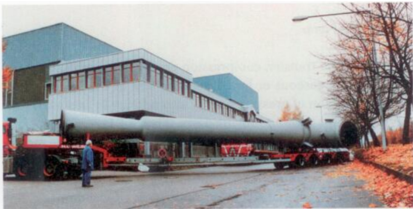
Figure 4.2 First stage of a steam jet vacuum pump for a steel degassing plant.
