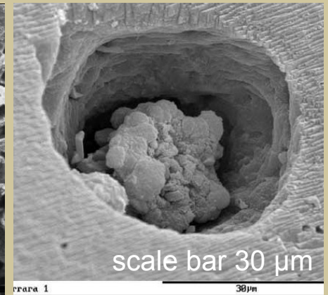
Fungal colony in a hole it etched into the marble.
