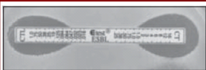
Figure 4. Clear cut ESBL positive: MIC CT/CTL = 1.5/0.047 = 32
