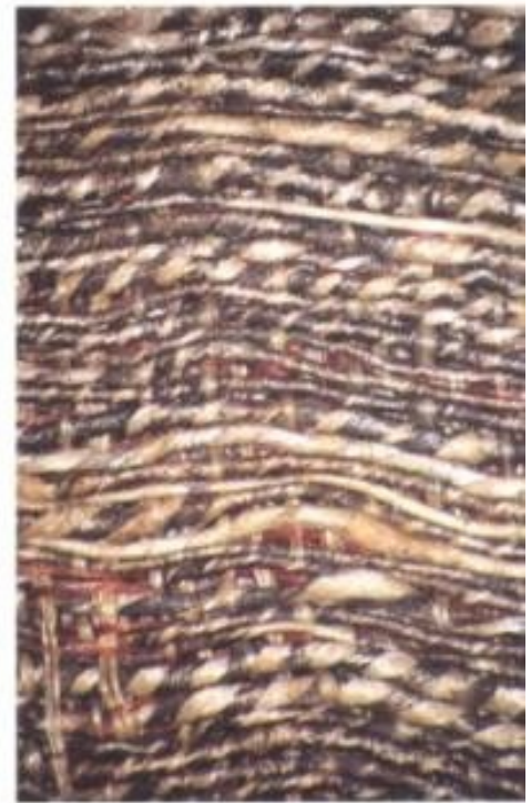
Fig. 5 Gew 370: Silver coated mem- brane strip wound around a linen core
