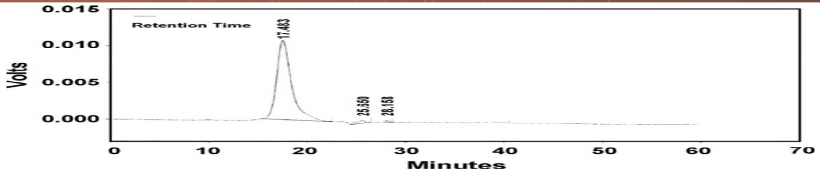
Fig. 5. HPLC analysis of purified F(ab)_2 . Elution profile of F(ab)_2 as single homogeneous peak represents >99% purity of the product. Column: SEC, TSK Gel-3000 SWXL (TosoHass). Sample: 20 \mu l of purified F(ab)_2 ; eluent: 20 mM phosphate buffer in 150 mM sodium chloride solution, pH 7.2, Detection at 280 nm; flow-rate: 1 ml \text{min}^{-1} .
