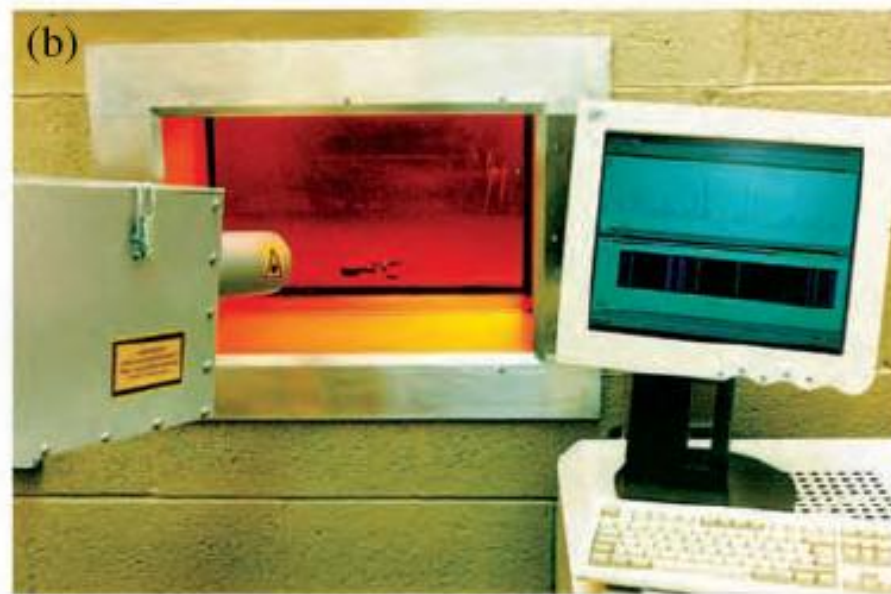
Plate 13 (a) Schematic showing the deployment of the remote LIBS instrument to monitor surface contamination. (b) Laser beam of the instrument being directed through the lead glass shield window (Applied Photonics, 2004a. Courtesy of Applied Photonics, Ltd) (see Figure 7.7)
