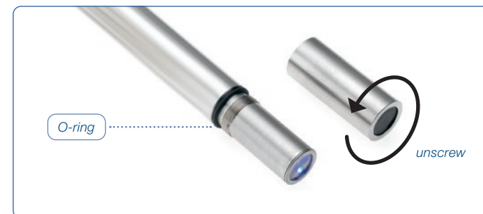
Figure 25: Replacing the ODO Cap of the VisiFerm DO Arc sensor
