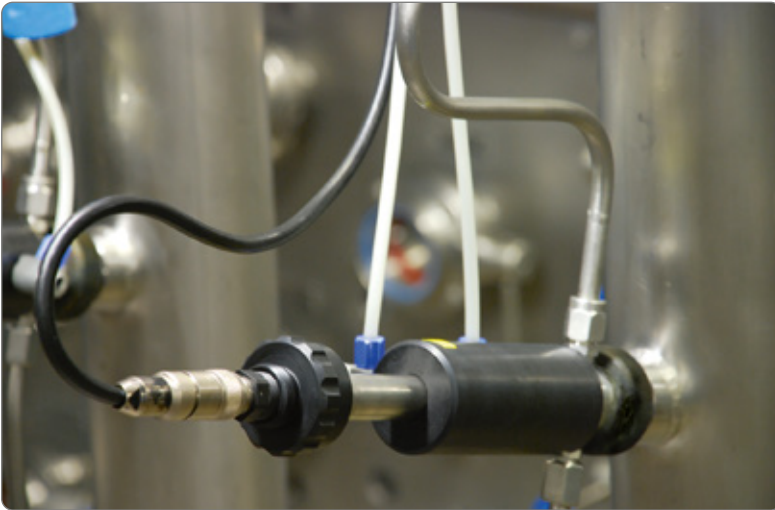
Figure 13. DO sensor in the wort line at Bitburger Brewery.
