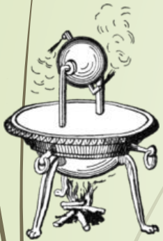
rudimentary steam engine was the aeolipile mentioned by Vitruvius between 30 and 15 BC
