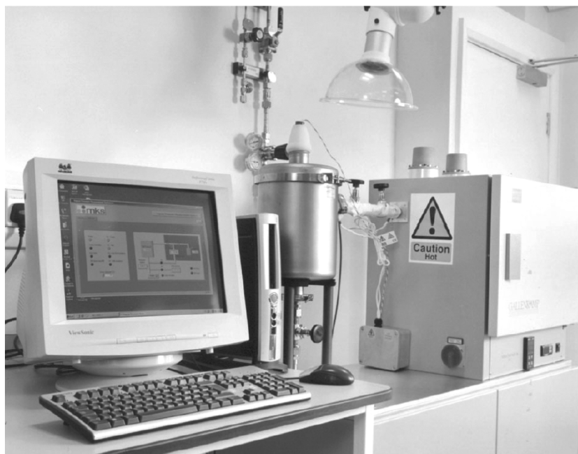
Figure 1.7 Apparatus used by a commercial manufacturer to accurately measure the vapour pressure of metalloorganic MOCVD and ALD precursors. (Reprinted from ref. 66, with permission from Elsevier.)
