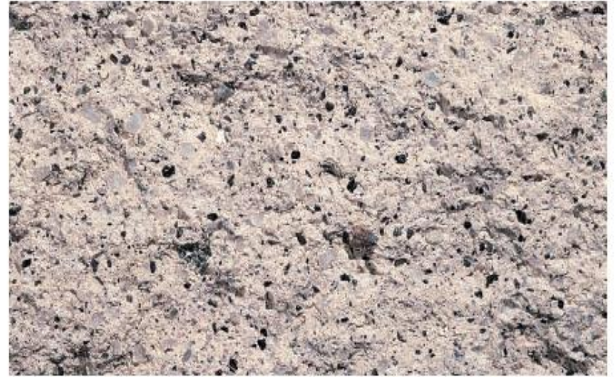
(B) Rhyolite: K-feldspar, plagioclase, quartz, biotite, and light-colored fine-grained groundmass.
