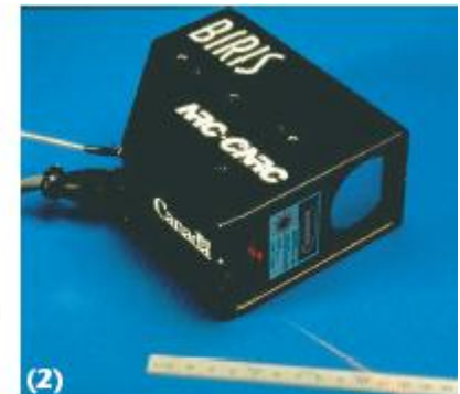
A Biris sensor. (1) The optical principle combines triangulation with a double aperture mask to improve the robustness of the laser line detection. (2) The head is compact and rugged. 10
