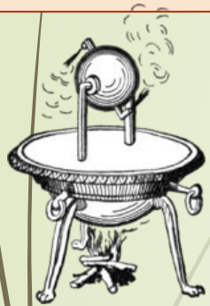
rudimentary steam engine was the aeolipile mentioned by Vitruvius between 30 and 15 BC
