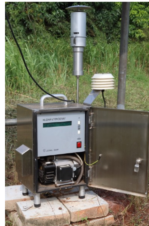
low volume active sampler MVS-6 (Sven-Leckel) - active sampling in Africa Ghana and Kenya since 2014
