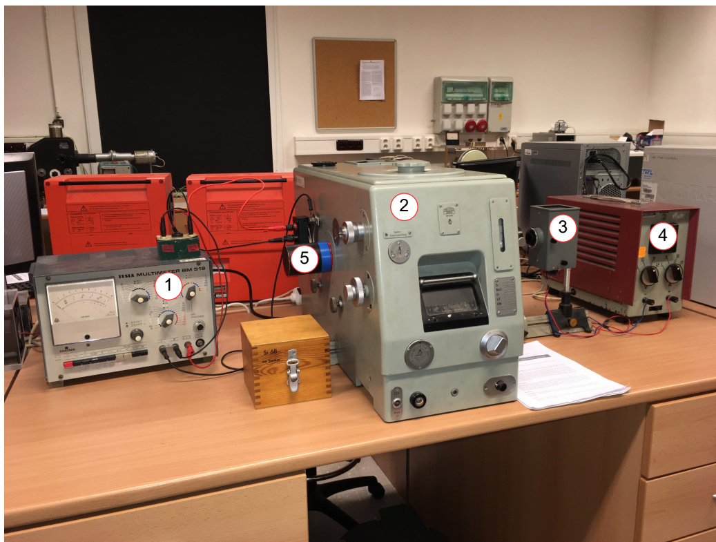
Figure 6: Measurement setup: 1 - Voltmeter, 2 - Monochromator, 3 - Lamp, 4 - Lamp voltage source, 5 - Photodiode cover.
