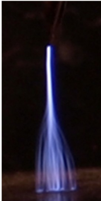
Figure 3. Photograph of TS in positive needle–plane gap of 4 mm, f = 2 kHz, R = 6.6 M \Omega and exposure 0.05 s.
