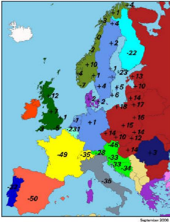
Figure 6: Differences between EVRF2000 zero level and the zero levels of national height systems in Europe (in cm)
