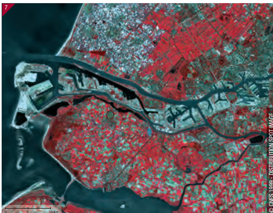
Satellite view of the port of Rotterdam. In this image, vegetation is shown in red and built-up areas in blue (image by SPOT 5).
