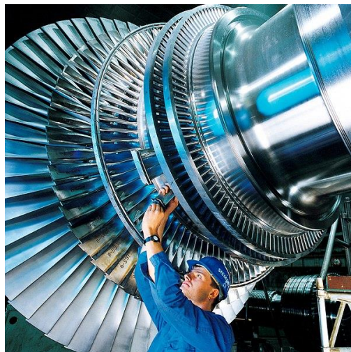
Siemens Pressebild, A worker installing a turbine blade on a steam turbine rotor being assembled in a Siemens factory in Germany. (online). (cit. 30.4.2024). Dostupné z: https://commons.wikimedia.org/wiki/File:Dampfturbine_Laeufer01.jpg GNU Free Documentation License
