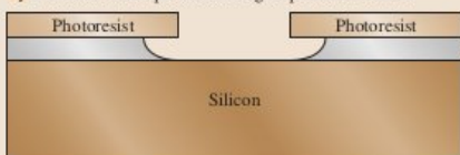
a) Profile for isotropic etch through a photoresist mask
