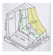
Lines = cuts through the p-V-T surface for fixed  $T \Rightarrow$  relationship between p and  $V_{\rm m}$  (molar volume).
